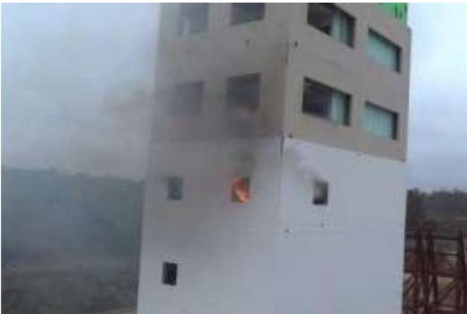
*Flames shoot from the five-story test building during WPI's post-earthquake fire tests. (Credit: Image courtesy of Worcester Polytechnic Institute)*
